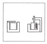
We do not recommend covers over the tracks. They can restrict part movement and make removing bent parts difficult. Rather than covers, it is better to design tracks using round rod or a thin blade as a **hold down** to maintain part orientation.
