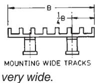
**Wide Tracks** – Two In-Lines in parallel, or side-by-side, are the solution when the track is *short but very wide.*
