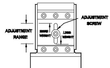
**NOTE: Do not overtighten the ADJUSTMENT SCREW** IF05.01
