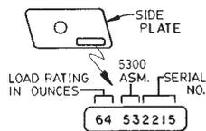
rating stamped on the In-Line's side plate?
