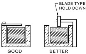
should be taken not to restrict part movement. Remember that the track is, in fact, moving up and down under vibration. The clearance between the underside of the cover and the top of a part is critical with regard to the
