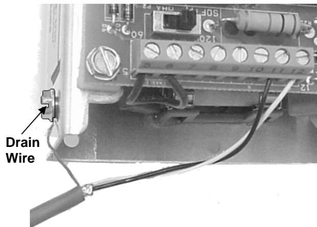
3. I/O wires within an enclosure should be routed as far away as possible from relays, solenoids, transformers, power wiring and other noisy equipment. Keep the I/O signal wires separate from the control's input and output power wiring. Secure the wires in place.
