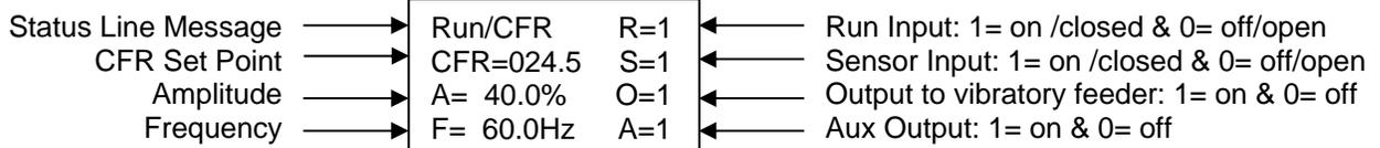
The normal operating display shows the status of the control with regard to input signals and control settings. They are listed from highest to lowest in priority. The highest priority message takes precedence over the other messages.
